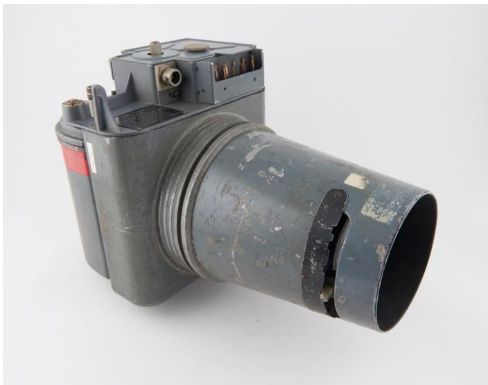
Figure 13 An air reconnaissance camera type F24, weight 8kg; the predominant kind used by the RAF during WW2; © The Board of Trustees of the Science Museum.
