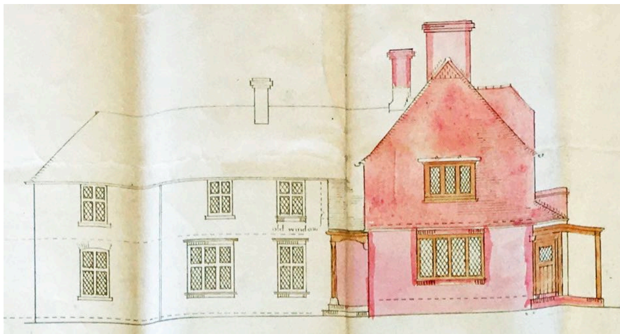
Figures 4b, c Two more views of the pre-existing structure at Slaters Oak from the 1907 planning application. In the details of the façades, the uncoloured parts are the original house and the pink ones are areas proposed for extension and re-modelling. One can see that the earlier house had a lower roof-line and was plainly built. The non-symmetrical layout of the windows in the older part shows that previous alterations had already been made. The new extension will have diamond-paned windows to match the older part. The façades of the most northerly range of the 'Z' were not affected by the proposals so not drawn, but according to the floor plans, this run incorporated a store room and larder off the kitchen, a stables and a coach house. Above, the west-facing elevation; below, the east-facing elevation.
