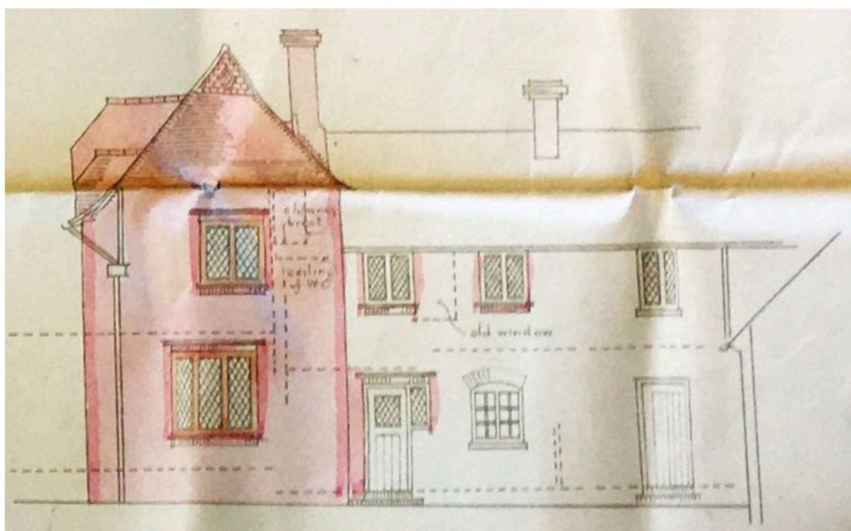
Figures 4b, c Two more views of the pre-existing structure at Slaters Oak from the 1907 planning application. In the details of the façades, the uncoloured parts are the original house and the pink ones are areas proposed for extension and re-modelling. One can see that the earlier house had a lower roof-line and was plainly built. The non-symmetrical layout of the windows in the older part shows that previous alterations had already been made. The new extension will have diamond-paned windows to match the older part. The façades of the most northerly range of the 'Z' were not affected by the proposals so not drawn, but according to the floor plans, this run incorporated a store room and larder off the kitchen, a stables and a coach house. Above, the west-facing elevation; below, the east-facing elevation.
